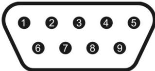
Pin 2: TX data: data transmission output
