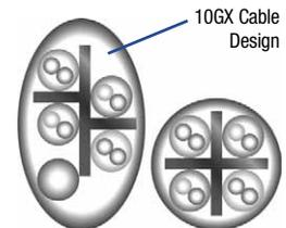
Since these features both increase and randomize the distance between a cable and its neighboring cables, both the ANEXT coupling and RL channel characteristics of the cable are improved. In fact, 10GX Cables were tested in a worst-case scenario – a six-around-one cable environment – and still exhibited performance well over proposed standards. In addition, this unique 10GX Cable design is more flexible and installer-friendly than other 10G cables.
