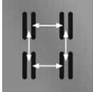
The IDC is one of the most sensitive areas for alien crosstalk management. In traditional designs, all of the IDC contacts are aligned so they become perfect antennas, allowing adjacent pairs to both emit and receive noise.
