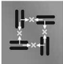
Belden's patent-pending design, called MatriX IDC technology, positions each IDC at 90 degrees to its neighbor – effectively canceling out ANEXT by 15 dB as compared with traditional technology!
