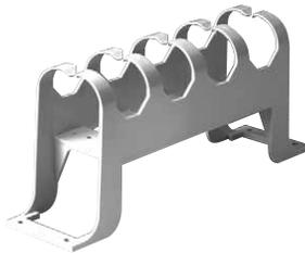
Wall mount cable management frames are pre-assembled vertical cable managers that are used between 110 wall mount frame kits for vertical management of patch cords. They simplify planning and installation of 110 cross-connect systems. They are available in two sizes to use with 300-pair and 900-pair wall mount frame kits.
